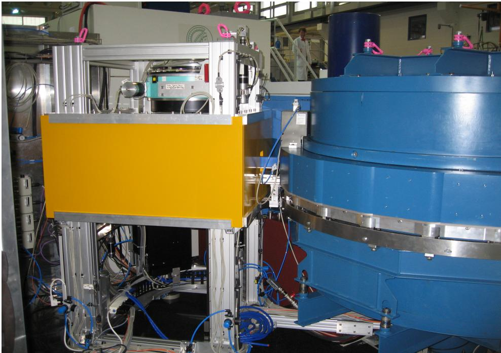
**Monochromatic single crystal diffractometer for large unit cells.**
