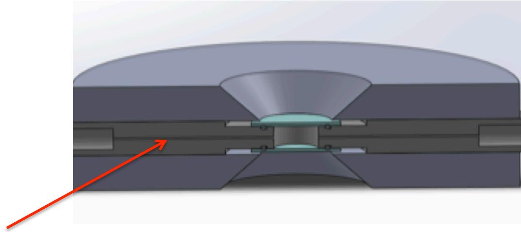
Two capillarity built in the spacer (0.5 mm diameter)
